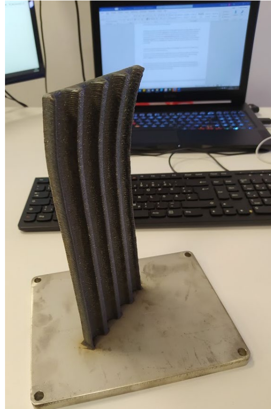
76% Scale Coil Positioning Plate Laser-Wire AM Test Print in 316-L Stainless Steel
