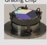
Titanium passively pumped vacuum package
