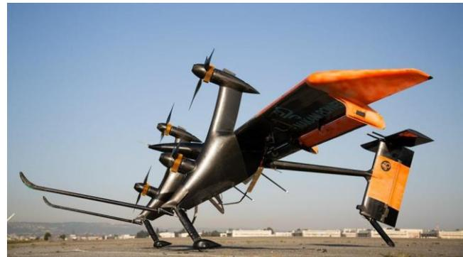
Figure 1: Makani's 20 KW (average output when flying under optimal conditions) working prototype
