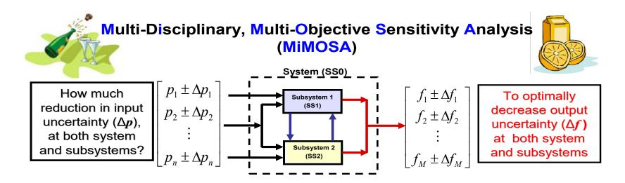
**Objective:** Optimally determine, with minimum investment (cost), the amount of uncertainty reduction needed in input parameters that results in minimum transmitted uncertainty in system outputs (or performance)
