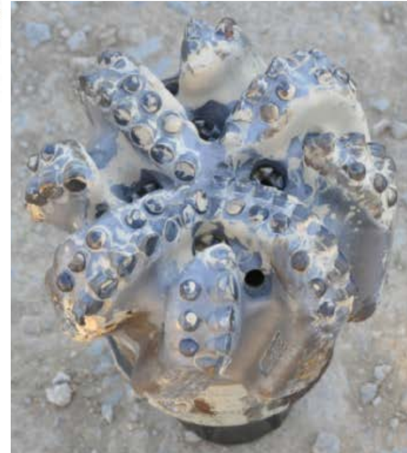
Worn bit after removal at ~2000 ft 3
