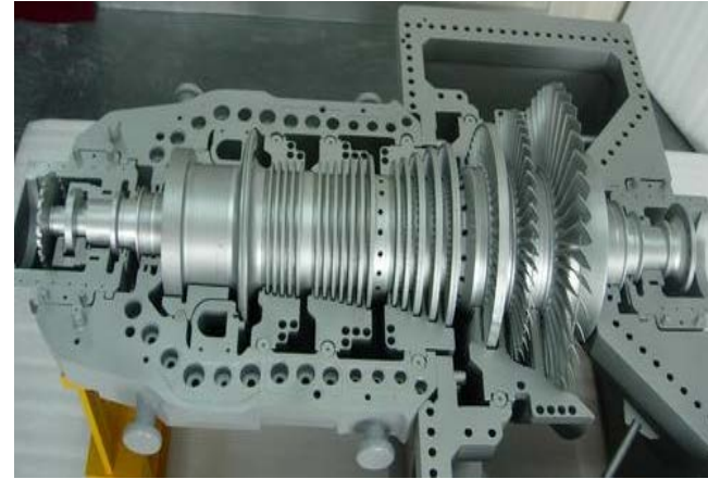
Steam turbine (50kW)
