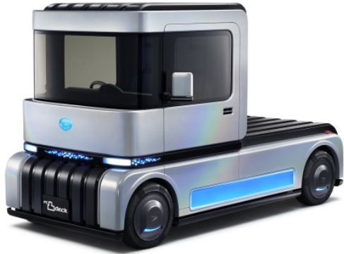
12 kW hydrazine hydrate fueled PGM-free AEMFC by Daihatsu Motor Co. www.electrical-cars.net
