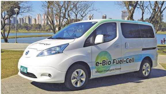
5kW ethanol fueled SOFC range extender (375+miles) by Nissan www.greencarcongress.com
