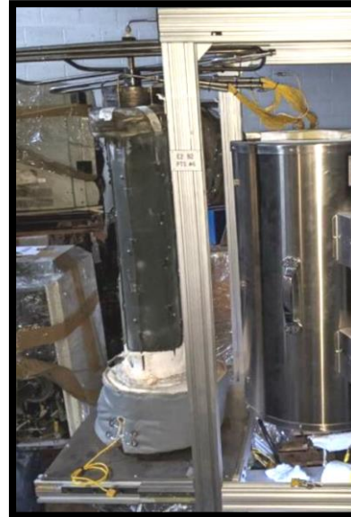
Pressurized Test Rig 7 Bar, 1.8 kW
