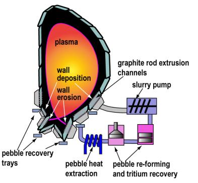
Provides increased resistance to any permanent wall damage from transients (disruptions, ELMs) and also provides faster recovery (startup) after these events.
