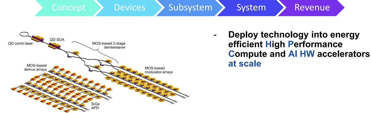
Following individual components to demonstrate >1 Tb/s, <1.5 pJ/b\* link have been fabricated and characterized: Laser, deinterleaver, modulator and SiGe APD\*
