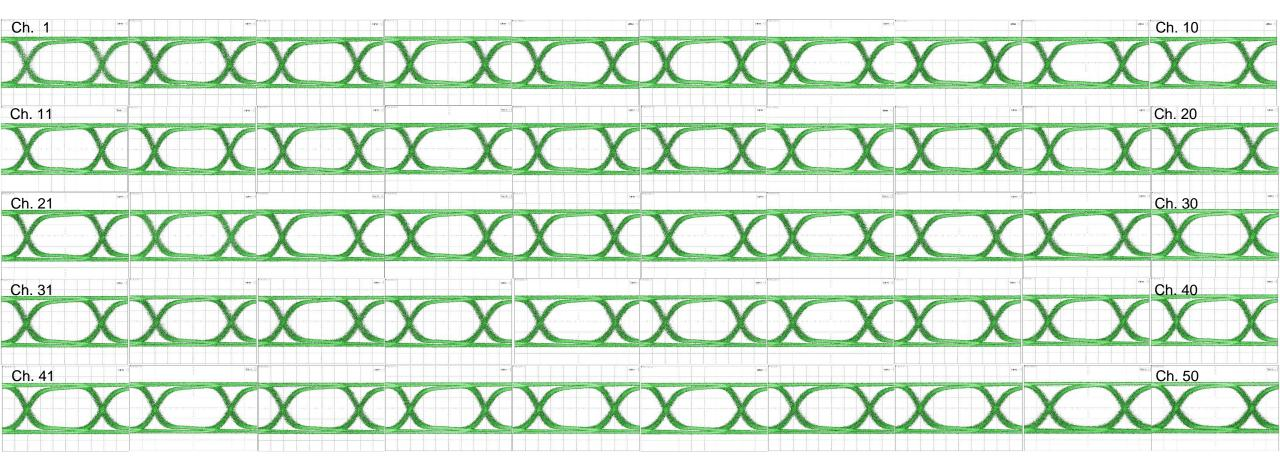
50 comb lines @ 10 Gb/s (setup limited) = 500 Gb/s with 509 mW laser power @ 50°C
