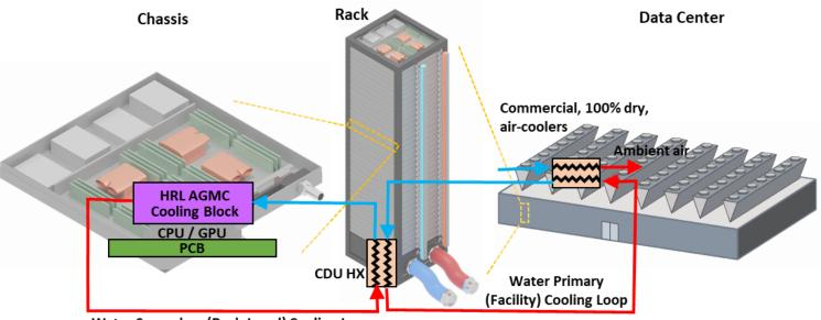
Water Secondary (Rack-Level) Cooling Loop
