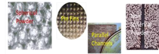
Potential heat transfer structures for PMCP
