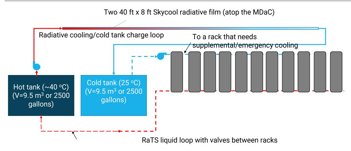
Mode 1- Direct cooling through radiative panels coupled to heat exchangers located within the datacenter Mode 2- with thermal storage- supplemental or emergency cooling to a rack from the cold tank (~1 hr)
