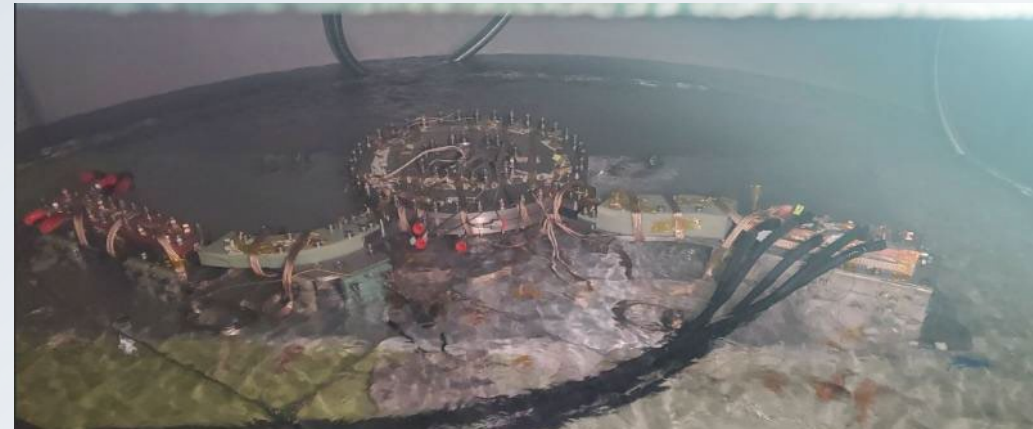
Aux coil during electrical testing in LN2
