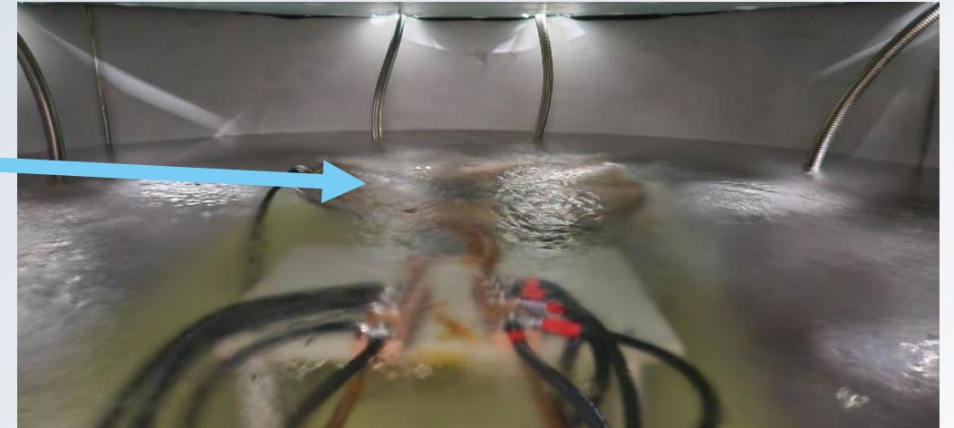
VIPER Jr coil during electrical testing in LN2
