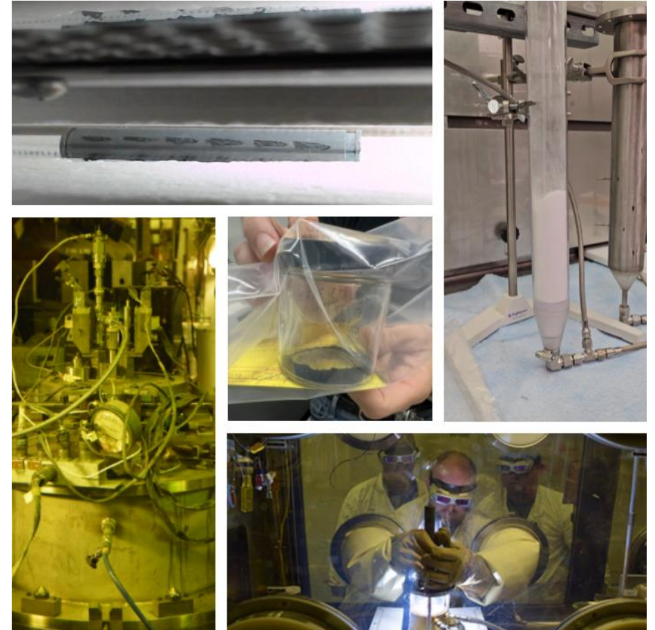
(Clockwise from upper left) Rodlet containing UO_2 pellets undergoing voloxidation. Fluidized bed. Electrowinning experiments. Lab-scale electrowinning. (Center) Sample of pulverized U_3O_8 from voloxidation.
