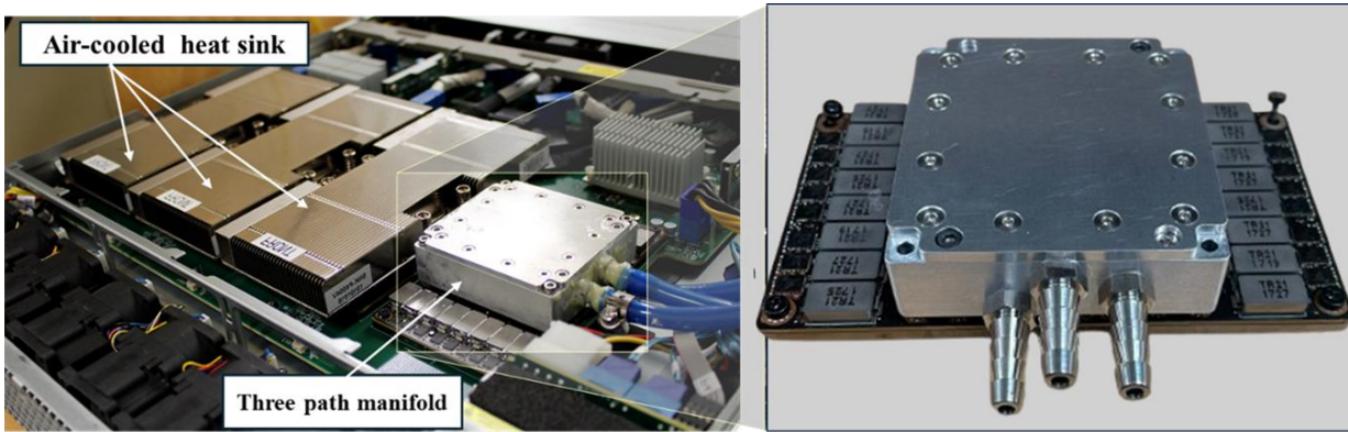
Integration of manifold with wick printed V100 GPU
