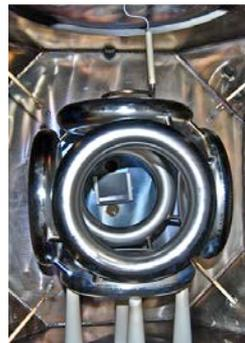
Since 1996, EMC2 has built and operated 19 test devices exploring magnetic confinement or Wiffle-Ball (WB) in the Polywell configuration, leading to a breakthrough in WB demonstration in 2013
