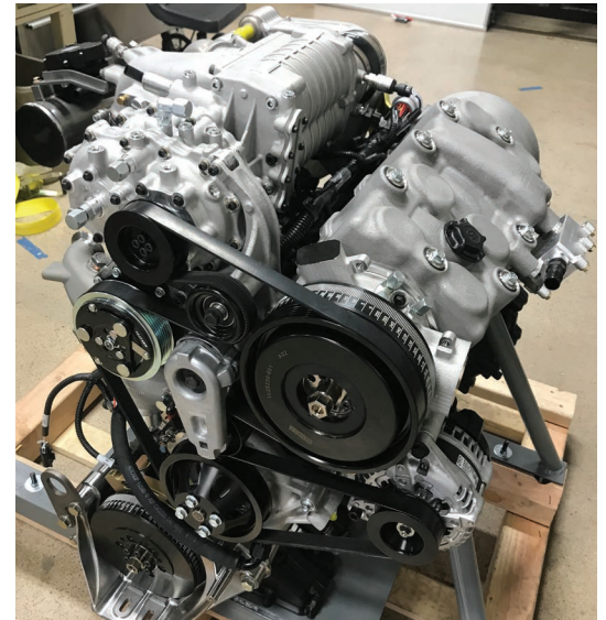
Figure 1: three-cylinder OP-GCI engine.
