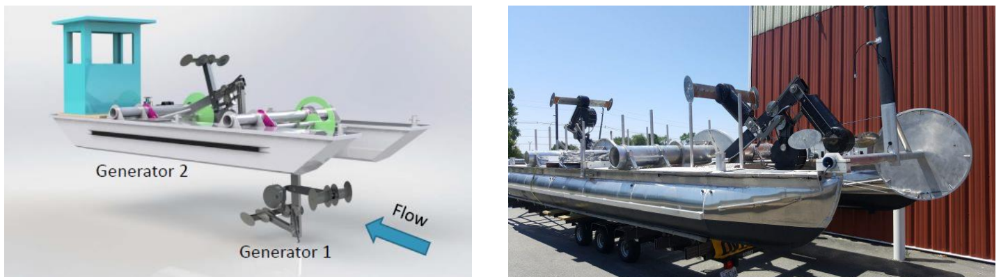
Figure 2: Brown University's 2kW prototype cyber-physical oscillating hydrofoil marine hydrokinetic energy generation system. (Left) Model of the floating platform design showing the generators, each with tandem hydrofoils, and their ability to pivot into and out of the water. (Right) Photograph of the fabricated device, before its multi-week deployment at the Massachusetts Maritime Academy.
