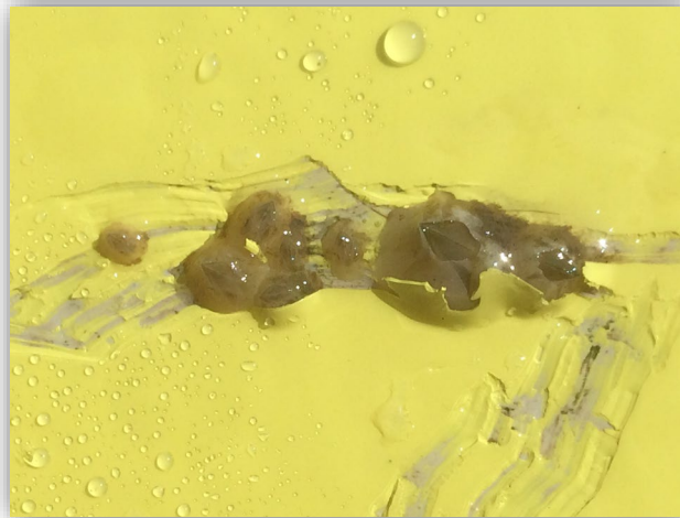
Damaged Coating Allows Barnacle to Adhere to Substrate
