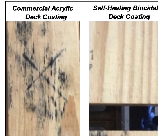
Localized Biocidal Activity at Damage Site
