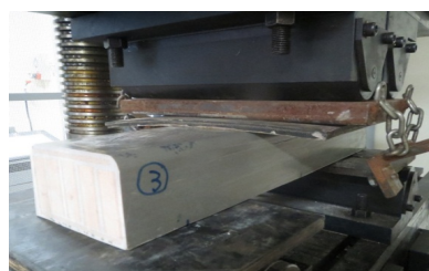
PF coated composite sleepers
