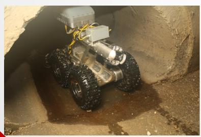
Drones are now being used for gravity pipe assessments in addition to aerial surveys
