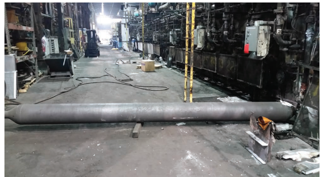
Figure 2: Furnace roll made with the ORNL team's alloy. This roll appears pristine after being in a plate austenitizing furnace at 900°C for 4000 hours. Compared to state-of-the-art alloy furnace rolls, the new rolls result in significantly lower maintenance costs and improved productivity.
