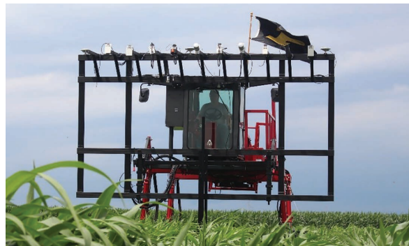
Figure 2 (left): The PhenoRover integrates visible, multispectral, ranging, and hyperspectral sensors. Figure 3 (right): Automated plant identification.
