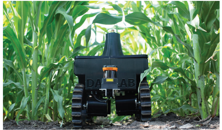
Figure 2 (left): One trial at UIUC. Ground robots collect sensor data from sorghum varieties at a rate of one acre every two hours. Figure 3 (right): TerraSentia is an ultra-compact 3D-printed robot.
