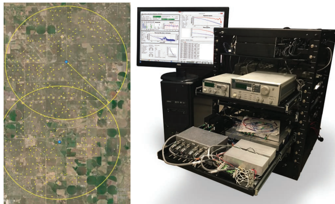
Figure 1: The CU-Boulder team developed a solution capable of monitoring hundreds of wellpads from a central location (left). The dual-comb spectrometer has been reduced to fit in a 19-inch, robust, and portable rack mount (right).
