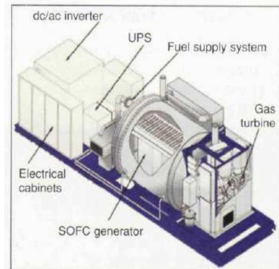
A schematic of the Siemens Westinghouse hybrid design. (Courtesy of Siemens Westinghouse)
