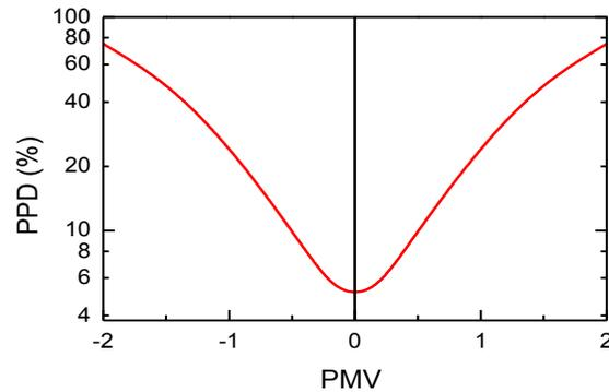
**Figure 2.** The PPD-PMV relationship based on Fanger's model<sup>6</sup>. Note: even at PMV of 0 which defines thermal neutral, the PPD value does not go to 0, reflecting the complexities of thermal comfort.
