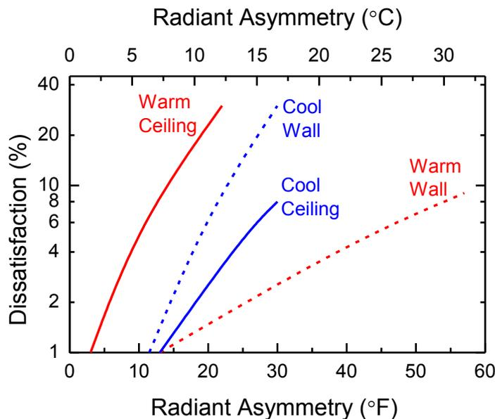
**Figure 4.** The percentage of occupants dissatisfied as a function of radiant temperature asymmetry. Note that the warm ceiling effect is the most undesirable, reflecting the disadvantage of overheating one’s head.
