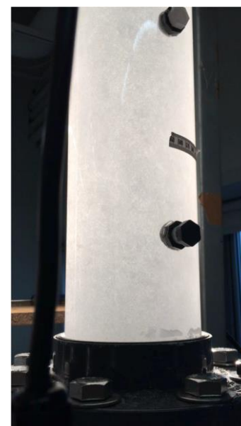
Figure 1: Picture of test reactor showing very fine bubble distribution
