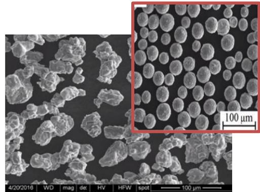
**Figure 1: Non-spherical HAMR TiH<sub>2</sub> powder vs. spherical GSD powder.**
