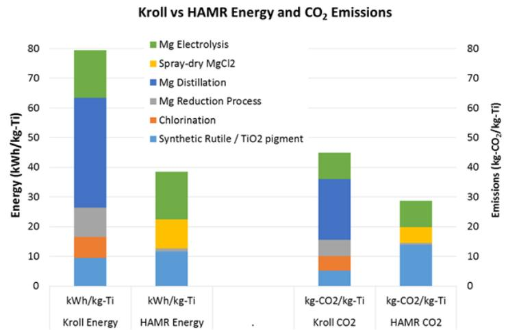
Figure 2: Energy and CO<sub>2</sub> benefits of HAMR vs. Current Ti Production Processes
