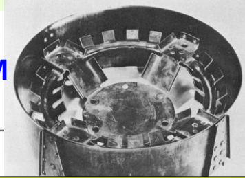
Ramjet Component (Hughes) TZM Mo Alloy (Mo-0.5Ti-0.1Zr)
